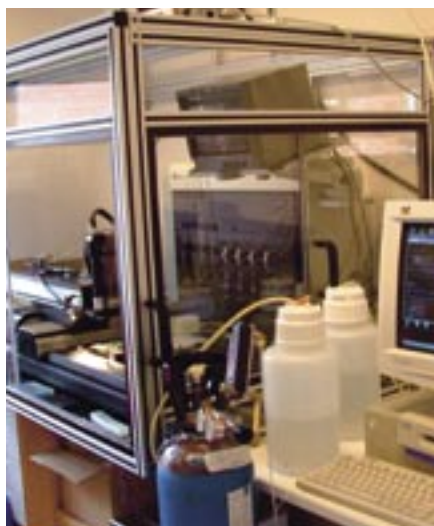
Here the researchers can portion out small volumes of 550 pL of antibodies for the production of microarrays.
